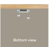
Install the strike plate under the top panel as indicated in the left illustration.
