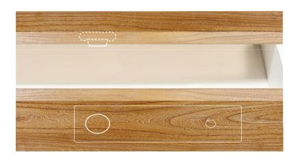
Measure and position where the loc-n-go and strike plate will be installed.
